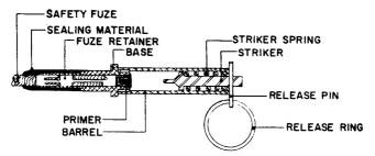
The attachment and operation of the M2 Fuse Lighter are as follows:
