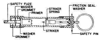
The attachment and operation of the M60 Fuse Lighter are as follows:
