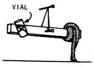
(2) Where no solvent is available or where the odor of solvent may make the device easy to detect, do not use cloth soaked with solvent. Use a wire basket containing ice as shown below.
