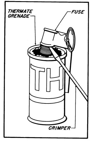
Fig. 61 — Defusing Thermate Grenade
