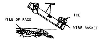
(3) When ice is used, the delay time will be a matter of minutes, depending on the ambient temperature. Ice cannot be used at temperatures near 32° F. Be sure that the drippings from the melting ice does not wet the igniter or interfere with initial combustion of flammable material.
