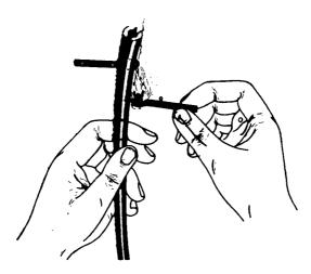
(f) Two standard fuse lighters, the M2 and M60, are available in demolition kits for positive lighting of Blasting Time Fuse and Safety Fuse M700 under all weather conditions—even under water if it is properly waterproofed. The devices are manually operated. A pull on the striker retaining pin causes the striker to hit the percussion primer, thus igniting the fuse. These devices are not recommended where silence is required because a report is heard when the primer is fired.
