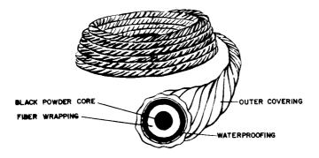
This consists of black powder tightly wrapped with several layers of fabric and waterproofing materials. It might be any color, orange being the most common. The diameter of this fuse cord is 0.2 inch (a little larger than  $\frac{3}{16}$ inch). This fuse burns inside the wrapping at a rate of approximately 40 seconds per foot. It must be tested before use to verify the burning rate.
